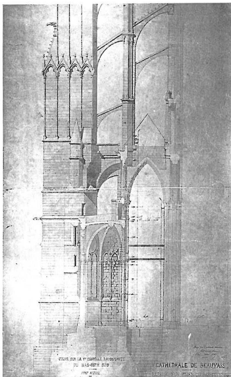
FIGURE 14. Drawing made for the restoration of pier F 8 by the architect Sauvageot in 1897 (MH. 201374).
