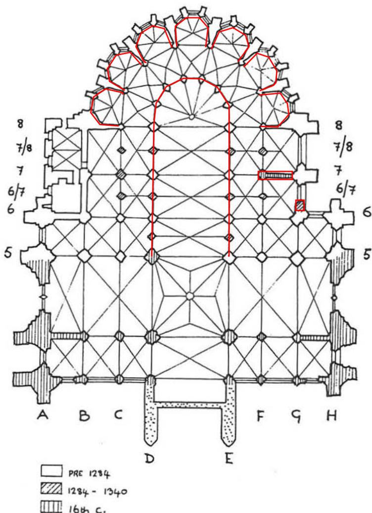
FIGURE 1. Plan of Beauvais Cathedral, showing repairs after the collapse.
