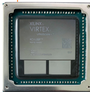
Xilinx VU35P with Dual-stack HBM2
