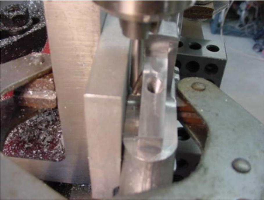
The first thing to do in this setup is the is the safety detent hole. Move back to 5.572" and off the center line by 0.295" and spot the location with a 3/16 center drill. Eyeball it with the safety hole as a double check before you drill 1/8" through. This detent is the headed variety and you must now drill a larger diameter for the head. Use a 5/32 drill, but be careful to only go 0.188" deep or you will be in bad shape.
