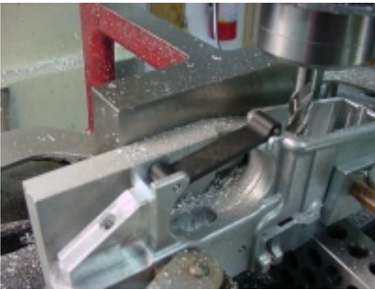
Always check your parts with the feature that is to receive them. I don't have to tell you it is a lot easier now to widen a tight slot than to find out later after you have anodized your work and the trigger guard won't fit!
