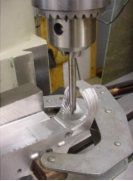
Since you will be drilling into the buffer tube threads, the investment in a long #3 center drill is well worth it. Move to the location and spot the hole to the full diameter (.250) of the center drill.
