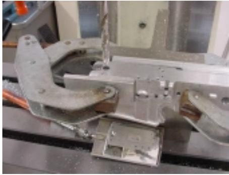
Next, put the 5/16" diameter hole through at the location shown below. This hole creates the little arc in the front of the mag well for clearance for the magazine rivits. This cut will leave a finished surface so feed lightly, use cutting fluid and clear the chips often. If you have a 5/16" reamer, then finish the hole with it.
