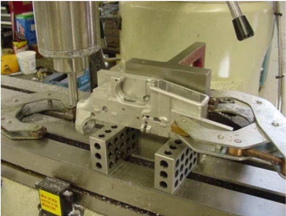
**Location:** Edge find the butt face and then add a second clamp once you have your spindle located. Move 7.500" and set your X axis zero over the pivot pin hole. Y axis zero should be the same as the last setup.
