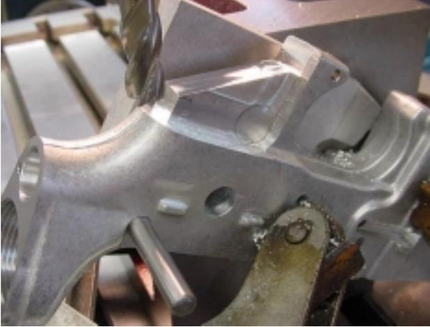
From the pin center-line to the surface to be milled is 1.228". Since we touched off on the top of the pin we will subtract the radius, .125" from the 1.400" giving us 1.103". Lower the table by this amount and mill the angle face of the pistol grip mount.
