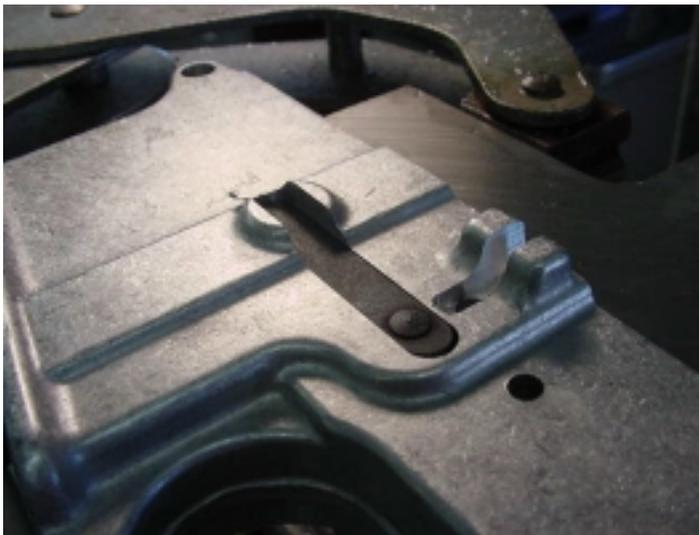
Go ahead, drop the magazine release in place. It should be close to flush with the reference surface. When you stop smiling, we can get going with the pistol-grip pocket.
