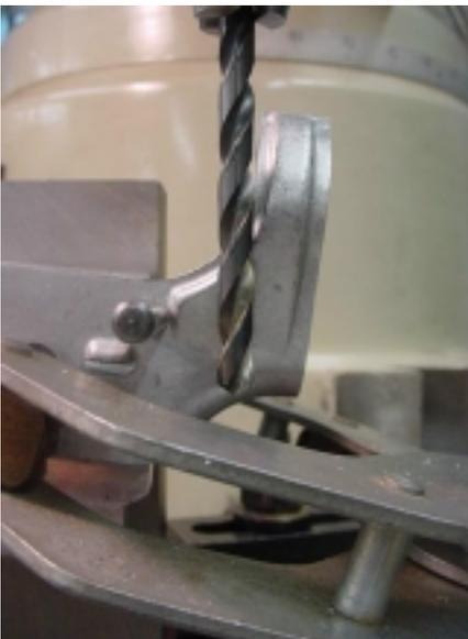
You don't want to make a mistake here by drilling through by accident. Double check your depth setting by moving to X-zero and bring the drill down to the stop and look in to see; first-that the drill tip will not break out of the forging at the bottom and second-that your drill chuck will not run into the top of the buffer tube ring.
