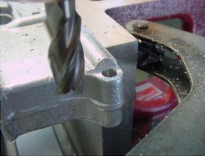
Now use a 3/8" cutter and move to 0.043 x (to the right of the pivot pin hole) and mill off the face at a setting of 0.522 from the centerline. Check that the pivot pin fits nicely before moving on.
