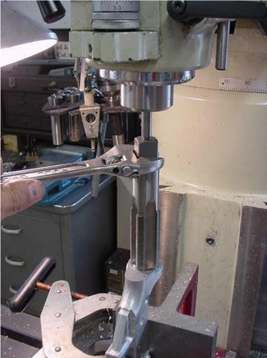
If you have the 1-3/16 - 16 tap go ahead and tap the hole. Put a center in the spindle to keep the tap aligned and with a light pressure on the down handle turn the tap with a wrench. If you don't have a tap, you can single-point the thread in a lathe, see the appendix.
