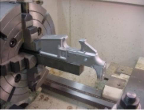
If you don't want to spring for the 1-3/16 x 16 tap for the buffer tube you can use the alternate method of cutting the thread by single pointing it in a lathe.
