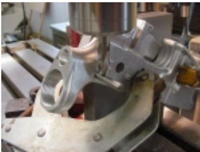
**Location:** Find the center line as usual and then put a .250 pin in the take down hole. Edge find the pin then move to its center and set zero. Chuck a 1/2" endmill and set the spindle stop and bring the spindle down and lock it against the stop. Raise the table until the cutter touches the pin and zero the elevation dial.
