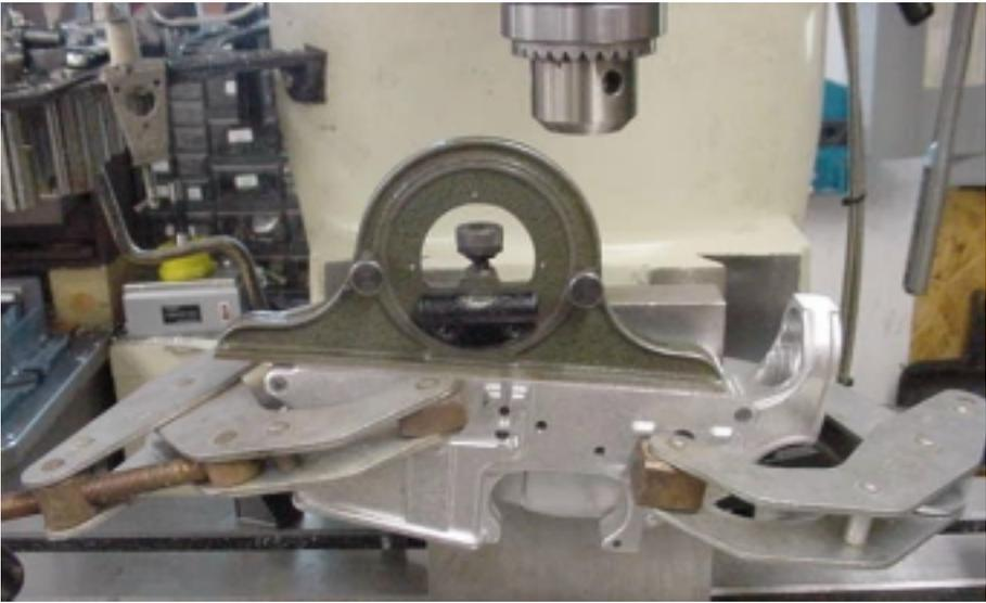
**Workholding:** Set your protractor for 6 degrees and clamp the forging against the angle plate using the clamping pad. Tap the forging until the bubble is level and add a second clamp. Re-check the angle after tightening the second clamp.
