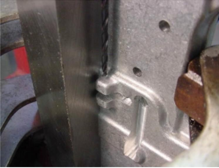
Locate the spindle at 0.625-.188 and chuck that long 3/32 drill. Here is where you will use that little block I told you to make in chapter one. Hold the block tightly against the angle plate and the forging. The drill should line up exactly with the hole in the block. Holding the block tightly, drill the hole through the lug on the forging. Drilling this hole any other way will drive you nuts!
