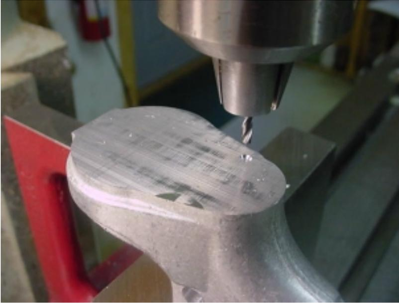
Next is the hole for the take down pin detent. Locate your spindle at 0.331-0.250 and drill a 3/32" hole down to the take down pin hole.
