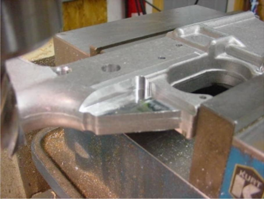
As in chapter three to cut the passenger side of the pistol grip mount chuck a 1/2" dia. cutter. No need to touch off, just take a light cut then measure the thickness and adjust from there for a finished size of 0.375".
