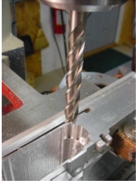
Initially, you may want to stay a few thousandths away from the finished size then take a second pass with the full length endmill to the finished dimensions shown below.
