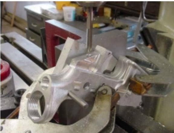
Chapter 7 check list. Check that all the features are completed before breaking your set-up.
