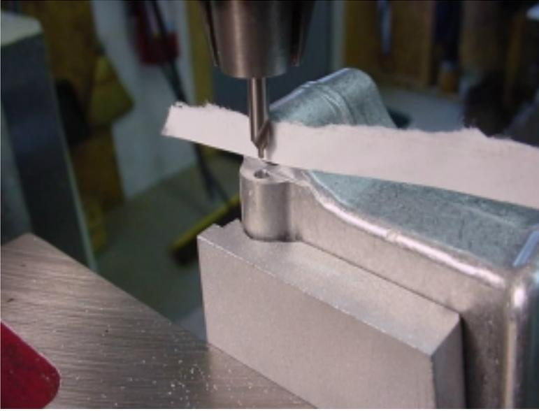
First in will be the pivot pin detent hole. Position your spindle at 0.000-0.583 and center drill with a #0 center drill. Choke a 3/32 drill and start the hole. Chuck the bit normally and finish the hole to 1.125" deep from the surface.
