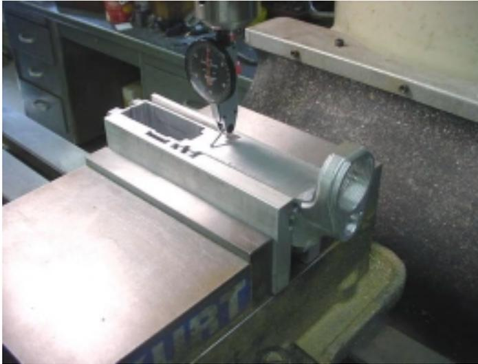
**Workholding:** Clamp up the forging and indicate it as in chapter nine. Position one clamp just behind and below the safety hole and the other clamp with a plate to protect the work just on top of the magazine release hole. Shown above is an alternate method using a machine vise. Clamp lightly and indicate the deck true then tighten the vise.
